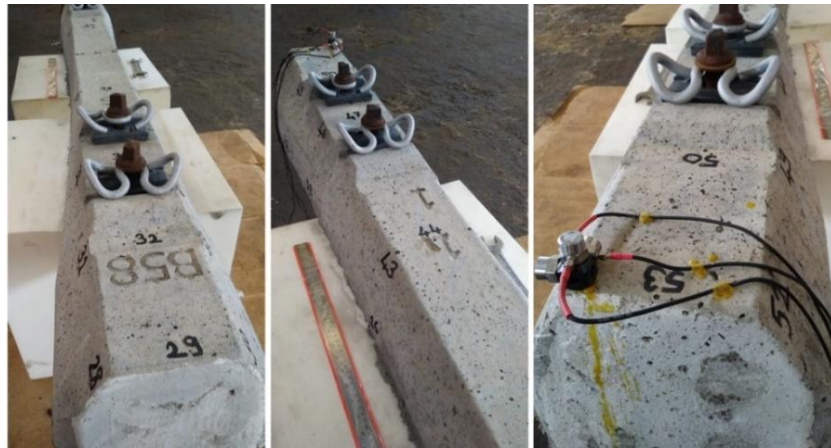
Figure 8. EMA test setup prepared for healthy and unused B58 type railway sleepers with fasteners
