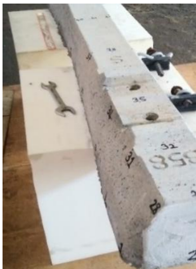
Figure 9. EMA test setup prepared for healthy and unused B58 type sleepers without fasteners
