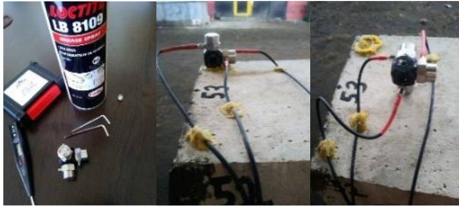
Figure 2. Accelerometer mounting details for three-axis EMA
